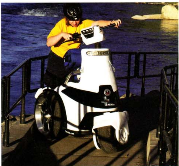
Logging a combined total of more than 100 miles on two T3s, crews test for maneuverability, turn radius and braking power.
