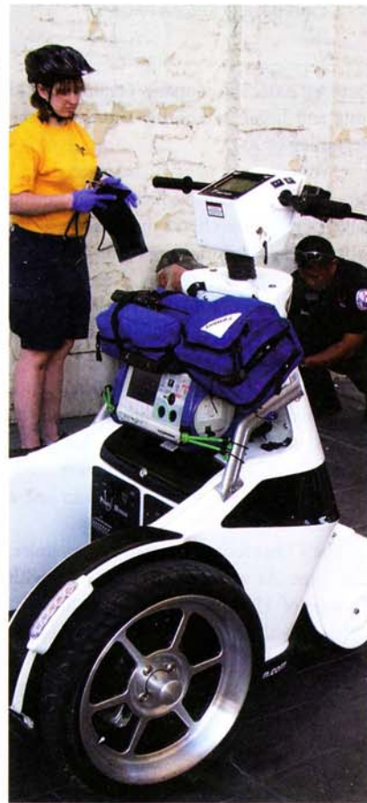
The large, lockable glovebox and shelf above the battery allows crews to carry equipment they would normally use on an ambulance.
